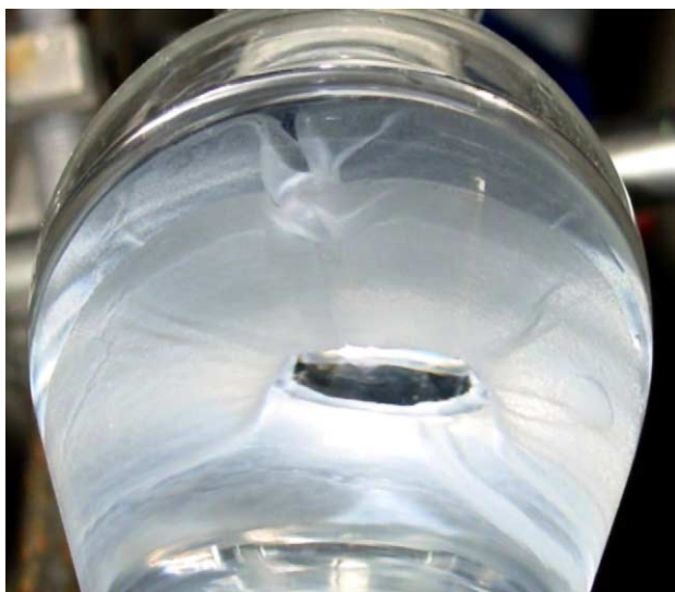
Fig. 8. The picture shows the layer of surfactant that accumulates at the octane–water interface when back-extraction of the encapsulated enzyme in the absence of stirring is attempted.
